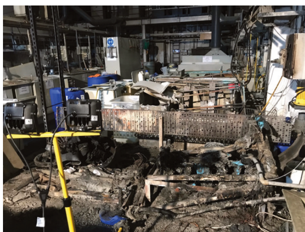
Image 1. Localised thermal damage with resultant smoke & water contamination
